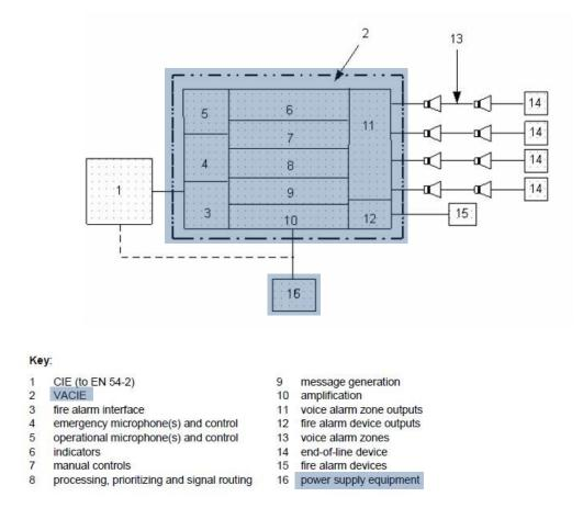
Figure 1: Components of voice alarm control and indicating equipment; source: EN 54-16:2008-06
